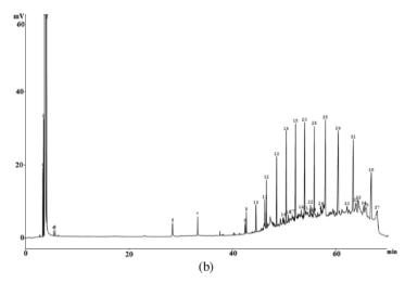
**Figure 4.** The chromatogram of initial condition sample (a), the chromatogram of sample after dissolved with bio surfactant of *P. citronellolis* bacteria with carbon source concentrations of 10% molasses (b)
