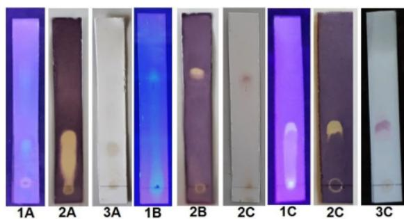
Figure 5. TLC-antioxidant bioautography; DJS1<sub>11</sub> (A), DJS2<sub>4</sub> (B), and BJS4<sub>2</sub> (C); in UV light 256 nm (1); sprayed 0.2% DPPH (2); sprayed 10% H<sub>2</sub>SO<sub>4</sub> (3)
