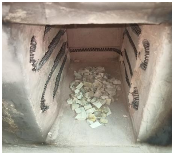
Gambar 17 Proses kalsinasi alat Furnace
