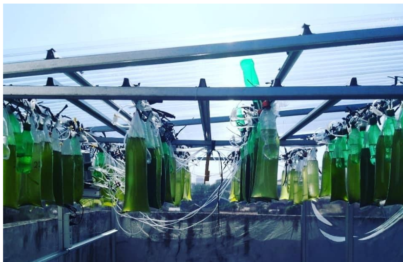
Fig. 3. Simple Photobioreactor model for microalgae culture
