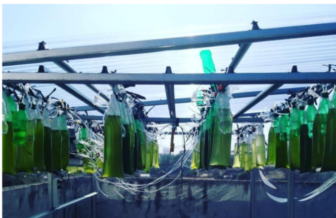
Fig. 3. Simple Photobioreactor model for microalgae culture
