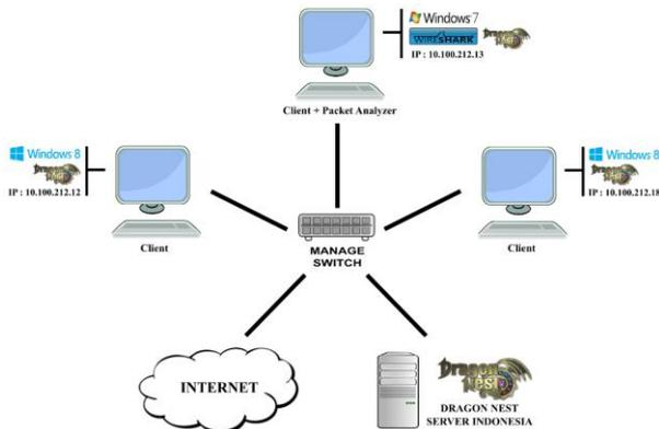
Figure 2. Testbed topology.
