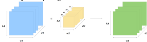
7 Gambar 2. Ilustrasi Convolutional layers Annual Research Seminar (ARS) 2019 Fakultas Ilmu Komputer UNSRI
