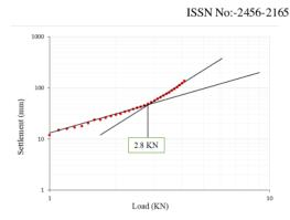
Fig 6:- Ultimate Bearing Capacity Using the De-Beer Method for the D06-20 Pile
