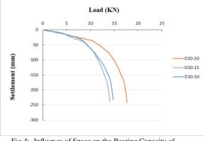
Fig 4:- Influence of Space on the Bearing Capacity of Helical pile
