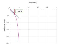
Fig 7:- Ultimate Bearing Capacity Using the Davisson Method for the D06-20 Test Object
