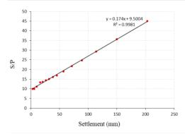
Fig 5:- Ultimate Bearing Capacity Using Chin Method for the D06-20 Pile
