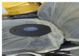
Source: personal documentation Figure 2 Accelerometer tool
