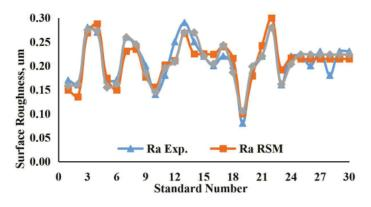
FIGURE 5. Surface roughness for experiment and predicted values
