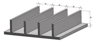
FIGURE 1. Geometry and dimension (mm) of the workpiece thin walled Ti<sub>6</sub>Al<sub>4</sub>V
