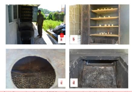
Figure 3. (a) Construction of neo-local WS Stove; (b) oven equipped with pin at the bottom; (c) grate for biomass bed and pot hole; (d) channel of flue gas from combustion chamber to chimney
