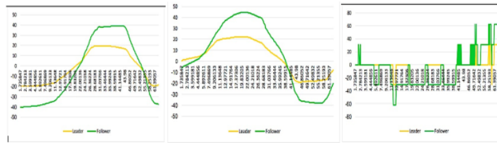
(a) The sample of PID response for x(t) , y(t) and \theta(t)
