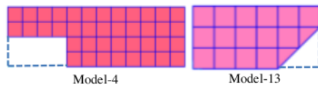
Figure 4. Buildings with subtractive results 10% - 15% in which their intact mass deformation behavior is symmetrical rectangles with two axes
