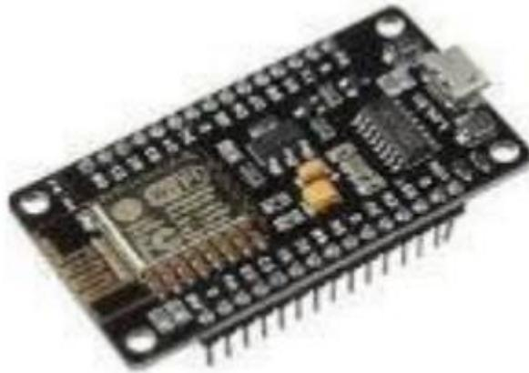
**Gambar 2.4** NodeMCU ESP8266 (Susantoi dkk., 2020).
