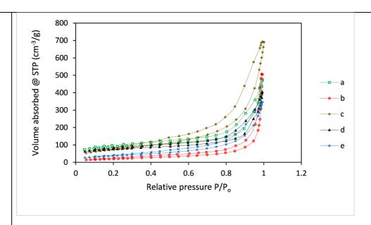
"Figure 5. N<sub>2</sub> physorptions of (a) SiO<sub>2</sub> (b) SiO<sub>2</sub>/Zr (c) SiO<sub>2</sub>-TEDTA (d) SiO<sub>2</sub>/Zr-TEDTA (e) SiO<sub>2</sub>/Zr-CEDTA"
