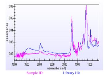
Fig. 6. Spectra of Non Imprinted Polymer (NIP)
