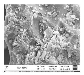
Fig. 3 Polymer before removal of simazine template
