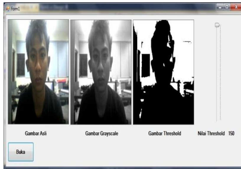
Fig 2. Conversion of the original image into a grayscale image and also to binary image with the threshold value of 150 in 8 bits.
