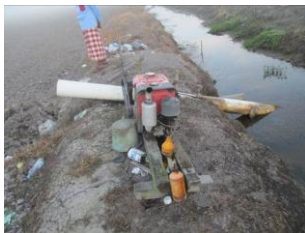
Figure 7. Pump irrigation on corn cultivation to elevate soil water table level.
