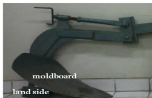
Fig. 2. The bottom of moldboard plow
