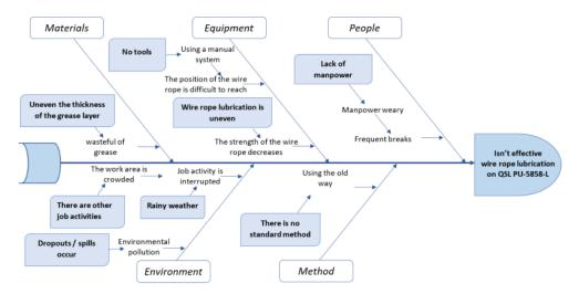
Figure 1. Analysis of fishbone diagram.
