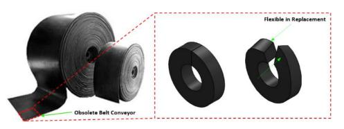
Figure 6. Reusable design of rubber seal of lubricator by obsolete belt conveyor
