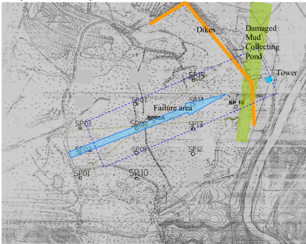
Figure 6 Layout of the boreholes
