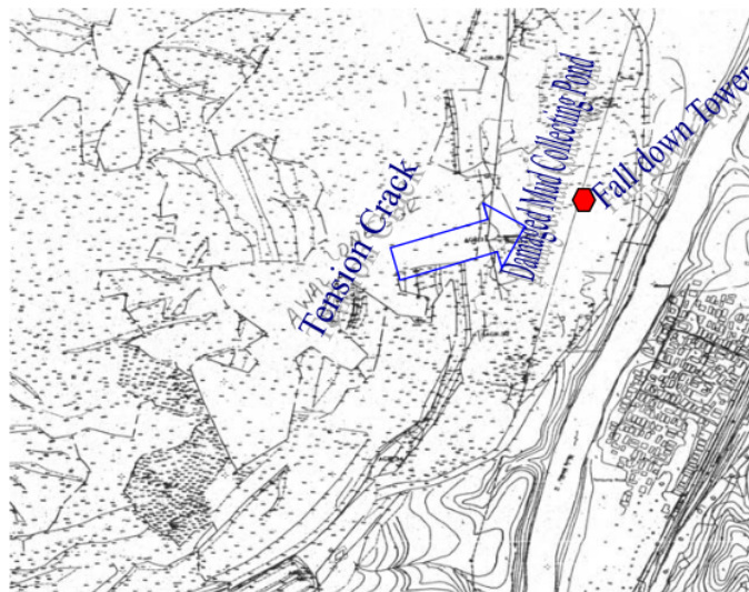
Figure 2 Situation of landslide
