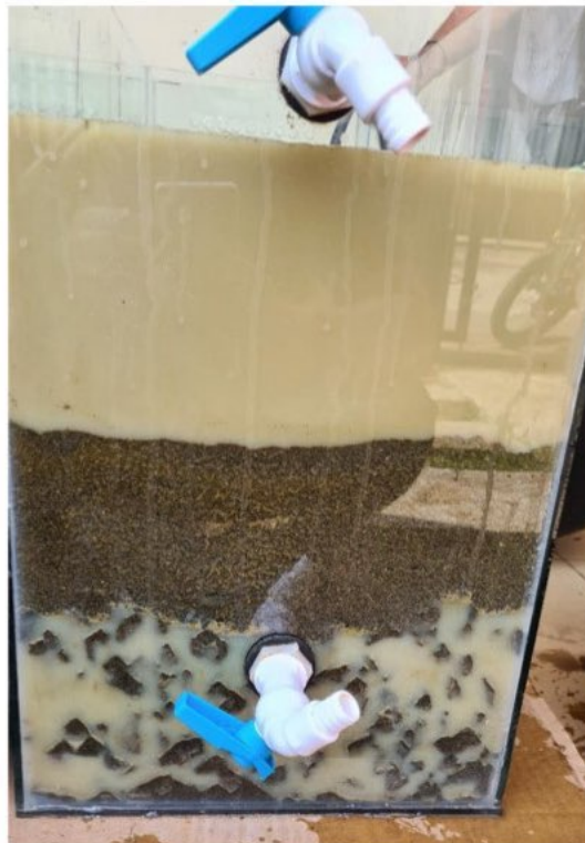
Gambar 4 Air Limbah Dimasukkan kedalam Constructed Wetland
