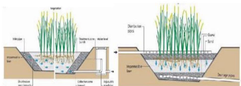
Gambar 2.2. (a) Tipe Horizontal SubSurface Flow; (b) Tipe Vertical SubSurface Flow (Morel & Diener, 2006)
