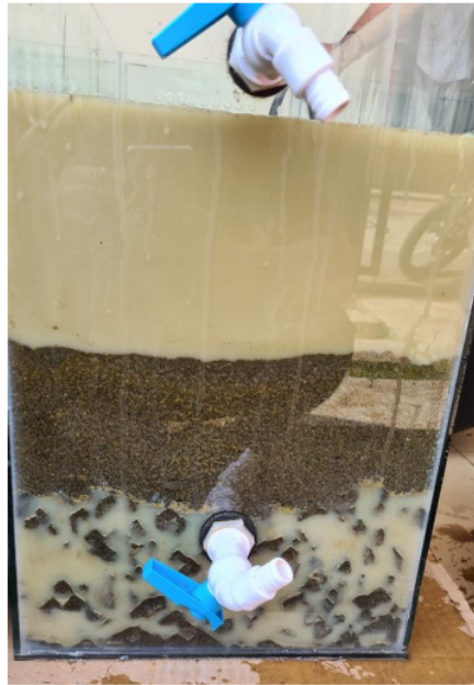
Gambar 4 Air Limbah Dimasukkan kedalam Constructed Wetland
