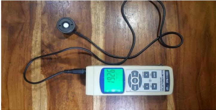
Gambar 5.9 *Solar Power Meter SPM-1116SD*
