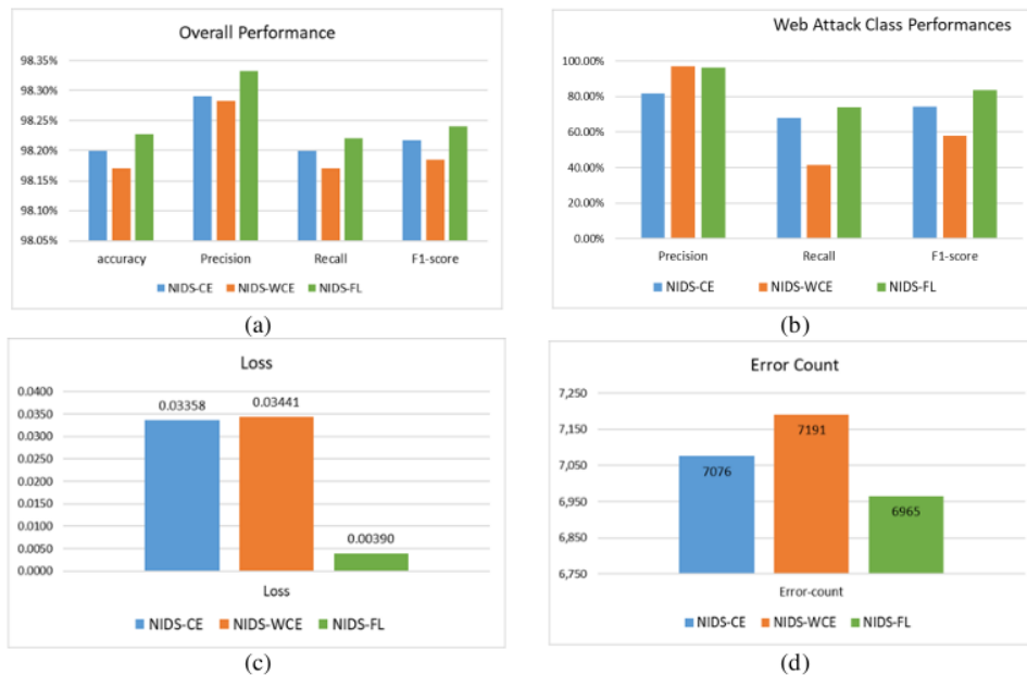
Figure 2. Graphs of comparison of various testing result metrics for all models (NIDS-CE, NIDS-WCE, and NIDS-FL) for the process epoch = 30; (a) Overall performance of attacks classification; (b) Performances of minority class-Web Attack class; (c) Loss value of all model; (d) Error count of all model
