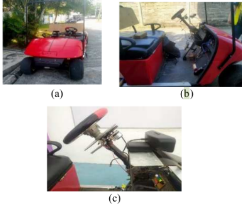
Fig. 3. Autonomous Electric Vehicle Front View (a), Side View (b), and Steering Control and Camera Location (c)
