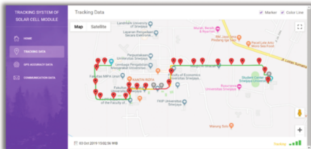
1 Figure 21.15 Visualization of coordinate data and the signal strength in real-time test of tracking system
