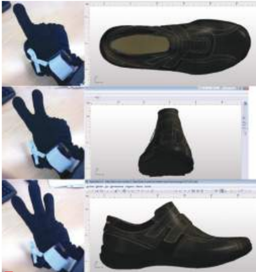
Figure 4.5 Glove gestures and the corresponding view [28]
