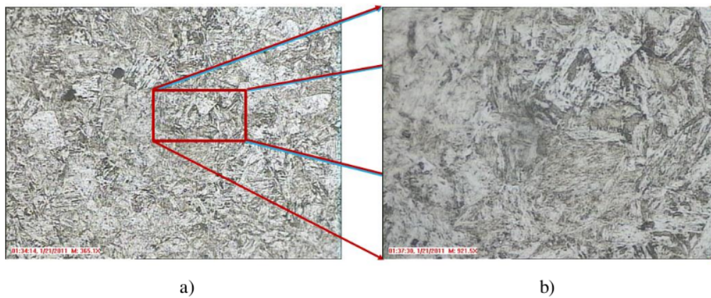
Fig. 8. Microstructure of failed link chain in the middle area
