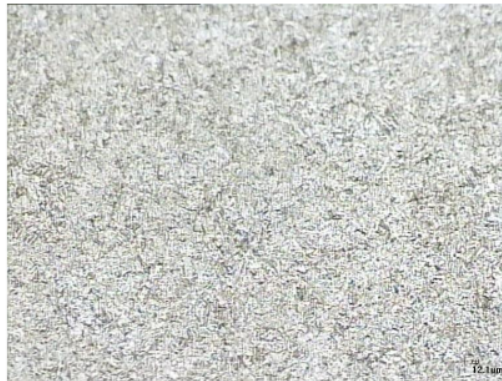
Fig. 10. Microstructure of as-received surface link chain in the middle area
