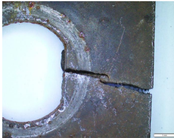
Fig. 6. Typically fractured chain link
