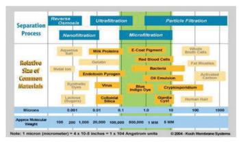
FIGURE 3. Classification of membrane filtration as a function of molecular weight cut off and pore size (Koch Membrane Systems).
