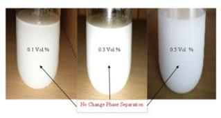
Figure 5. Photographs of TiO<sub>2</sub>/Virgin Coconut Oil Nanofluid at The Static Condition: Just After Preparation
