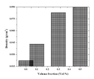
Figure 4. Density of Nanofluid at A Different Volume Fraction
