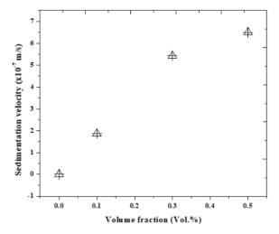
Figure 7. Sedimentation Velocity of  ${\rm TiO_2/Virgin}$  Coconut Oil Nanofluids
