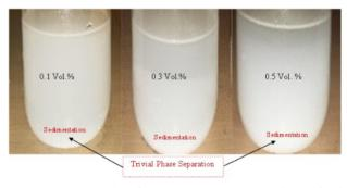
**Figure 6.** Photographs of TiO<sub>2</sub>/Virgin Coconut Oil Nanofluid at The Static Condition: Eight Days After Preparation
