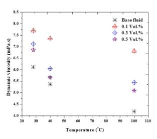
Figure 3. Viscosity of Nanofluid at Different Temperatures
