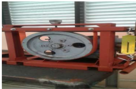
Figure.2. Prony-Brake Dynamometer coupled with engine flywheel
