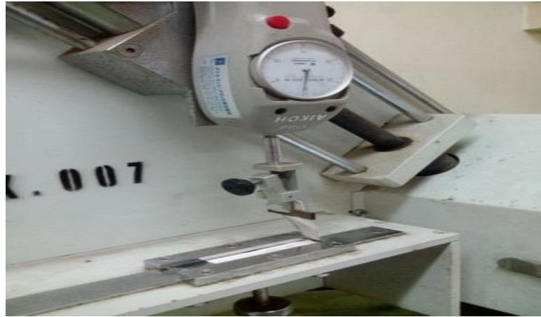
Figure 6. Process Polyvinylidene Fluoride membran tensile testing
