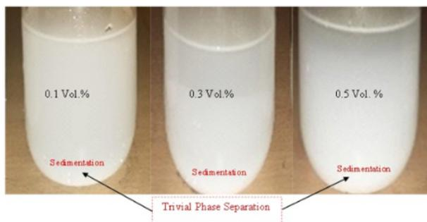
Figure 6. Photographs of TiO<sub>2</sub>/Virgin Coconut Oil Nanofluid at The Static Condition: Eight Days After Preparation
