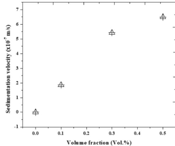
Figure 7. Sedimentation Velocity of TiO<sub>2</sub>/Virgin Coconut Oil Nanofluids
