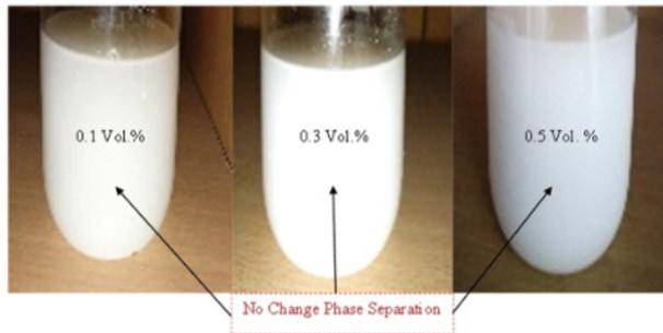
Figure 5. Photographs of TiO<sub>2</sub>/Virgin Coconut Oil Nanofluid at The Static Condition: Just After Preparation
