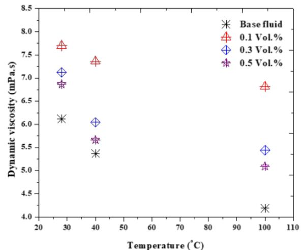
**Figure 3.** Viscosity of Nanofluid at Different Temperatures
