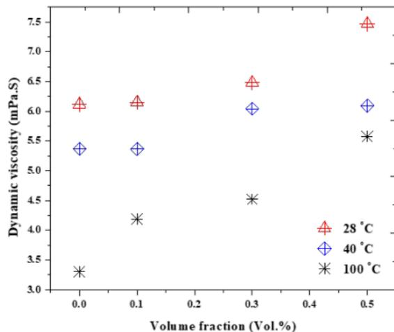
**Figure 2.** Viscosity of Nanofluid at A different Volume Fraction
