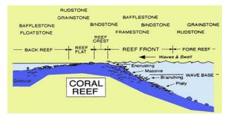
Figure 2. The Model Carbonate Facies [3]
