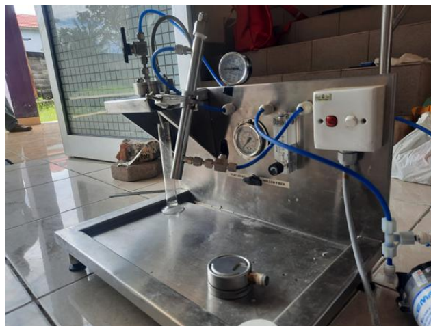
Figure 4. Clean Water Permeability
