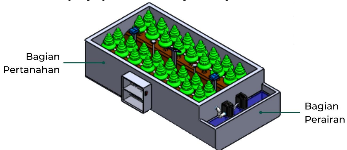
Gambar 2.1 Desain 3D Sistem Prototipe Plant Care
