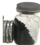
Figure 2. The Magnetite Nanoparticles exposed to the magnets
