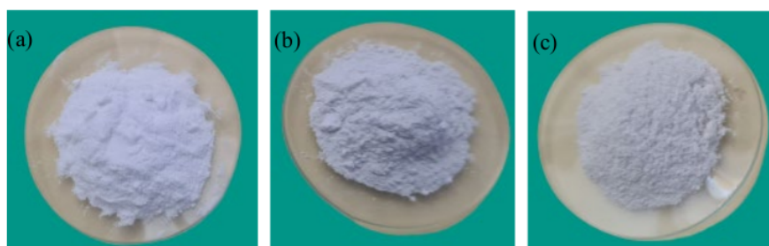
Figure 1. The silica extracted at a calcination temperature of (a)700°C, (b)800°C and (c)900°C
