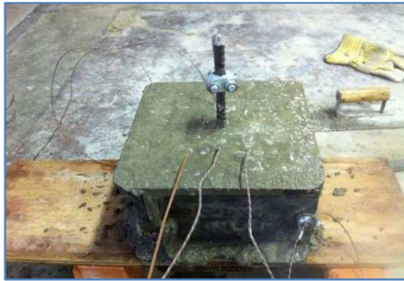
Figure 1 (a): Thermocouple casted into Concrete
