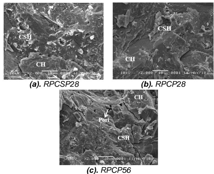
Fig. 10. SEM with  $w/c = 0.26$
