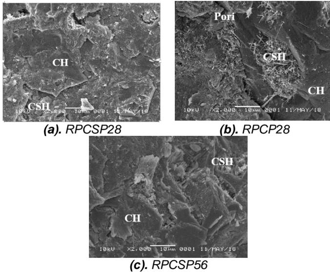
Fig. 8. SEM with  $w/c = 0.20$
