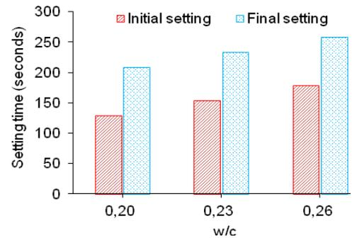
**Fig. 2. Effect of w/c on setting time**
