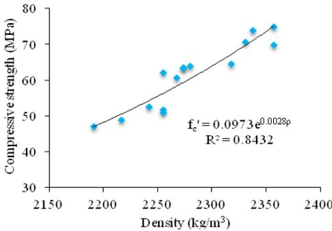
Fig. 5. Compressive strength vs density without sulfate immersion
