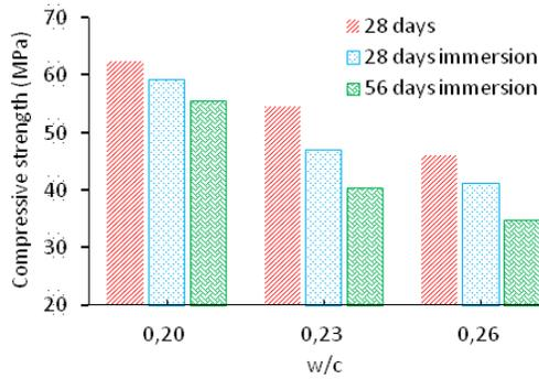
Fig. 4. Effect of w/c on compressive strength
