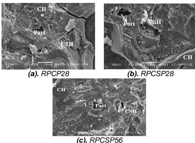
Fig. 9. SEM with  $w/c = 0.23$
