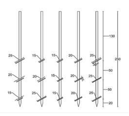
Fig. 1. Configuration of helical pile
