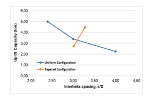
Fig. 9. The effect of s/D to uplift capacity
