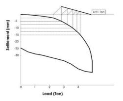
Fig. 7. The ultimate load estimation using Mazurkiewicz
