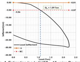
Fig. 4. Estimation load of U3S – 15 using Davisson
