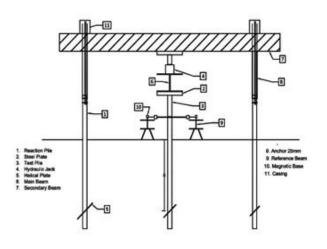
Fig. 2. Typical setup for uplift load test
