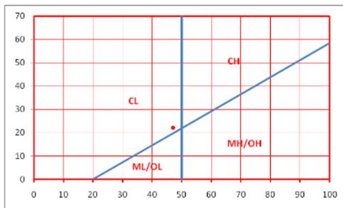
**TABLE 3-6 Classification of Soils and Soil Aggregate Mixtures\***
