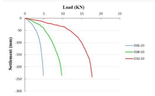
Fig 3:- Influence of Diameter on the Bearing Capacity of the Helical pile
