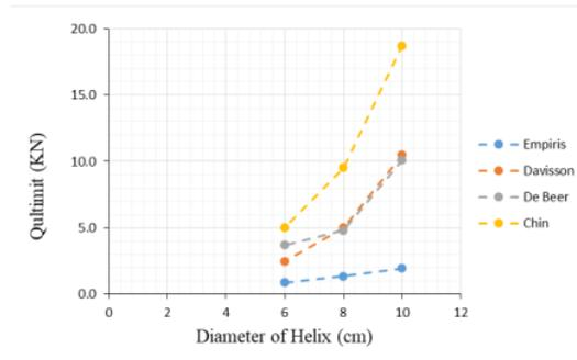
Fig 9:- Comparison of Bearing Capacity Value between Methods Due to The Influence of Diameter
