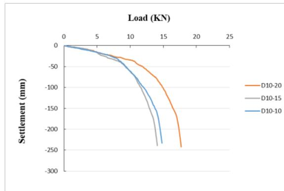
Fig 4:- Influence of Space on the Bearing Capacity of Helical pile
