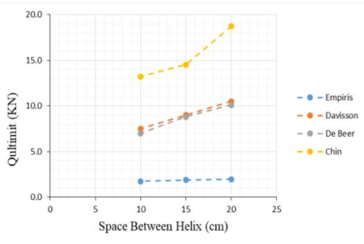
Fig 8:- Comparison of the Bearing Capacity Between The Methods Due to The Influence of Spacing
