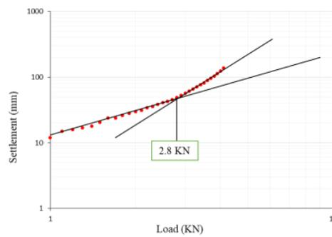
Fig 6:- Ultimate Bearing Capacity Using the De-Beer Method for the D06-20 Pile
