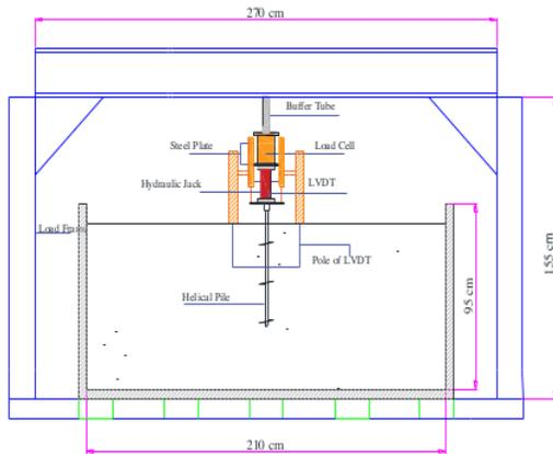
Fig 1:- Illustration of Testing Instrument
