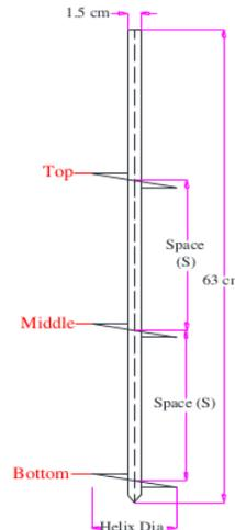
Fig 2:- Illustration of The Helical Pile
