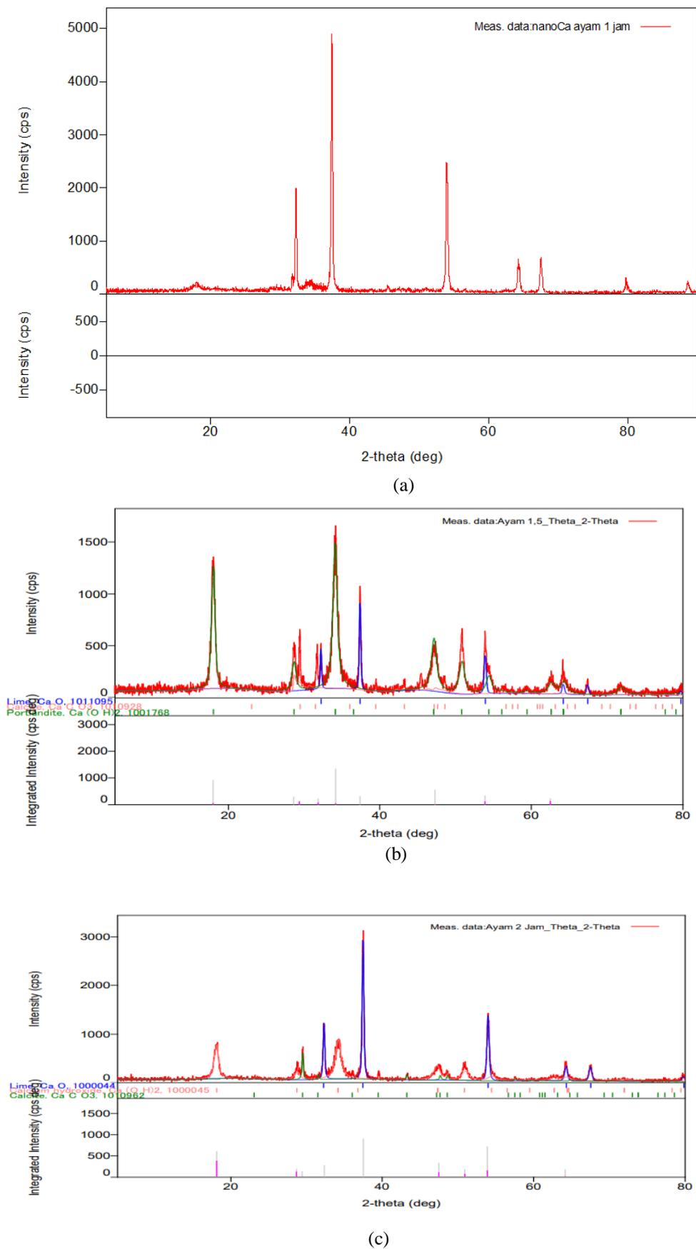
Figure 1 XRD of nanocalcium chicken eggshells from (a) 1-hour extraction, (b) 1.5-hour extraction, and (c) 2-hour extraction.
