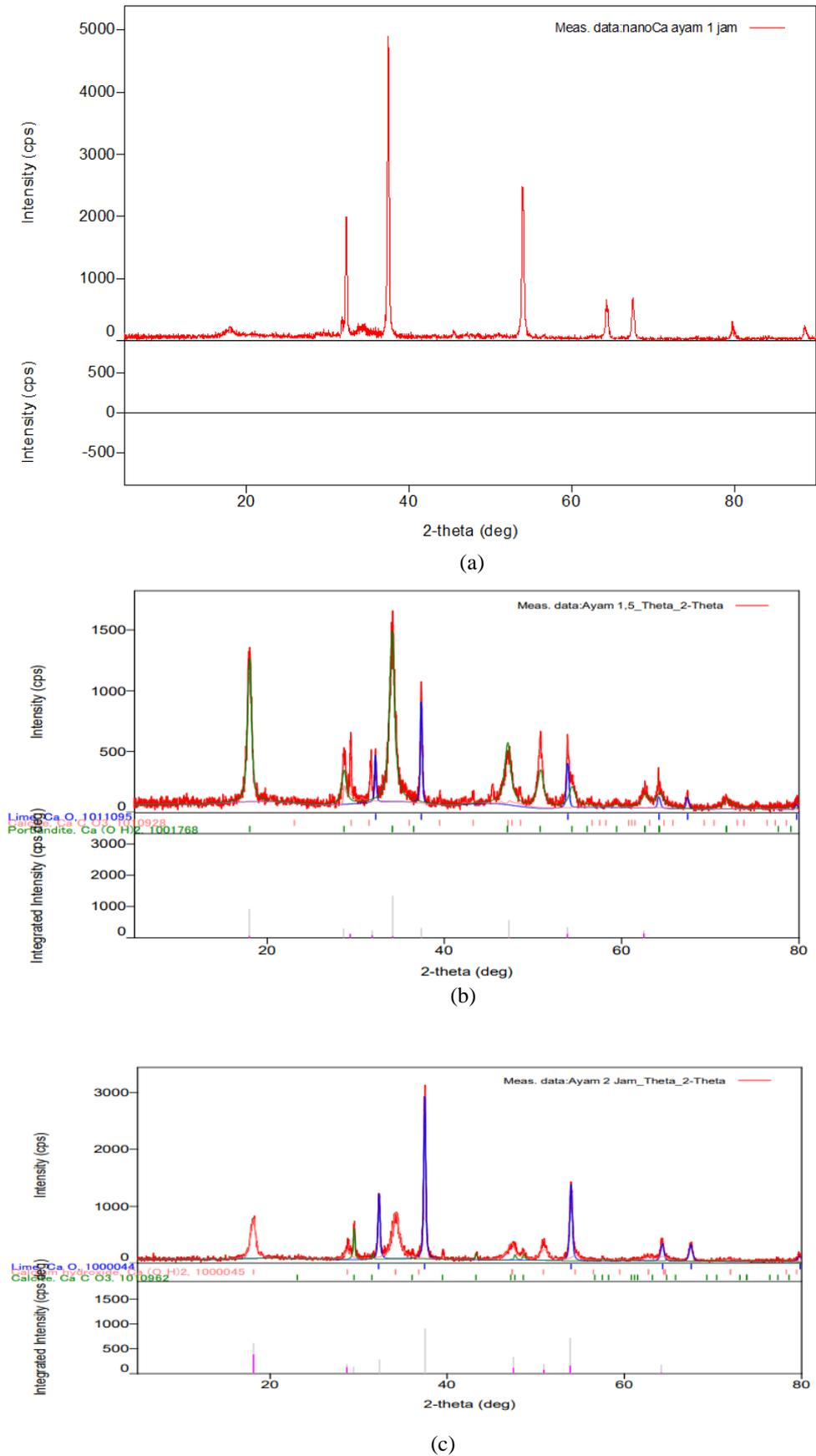
**Figure 1** XRD of nanocalcium chicken eggshells from (a) 1 hour extraction, (b) 1.5 hour extraction, (c) 2 hours extraction time
