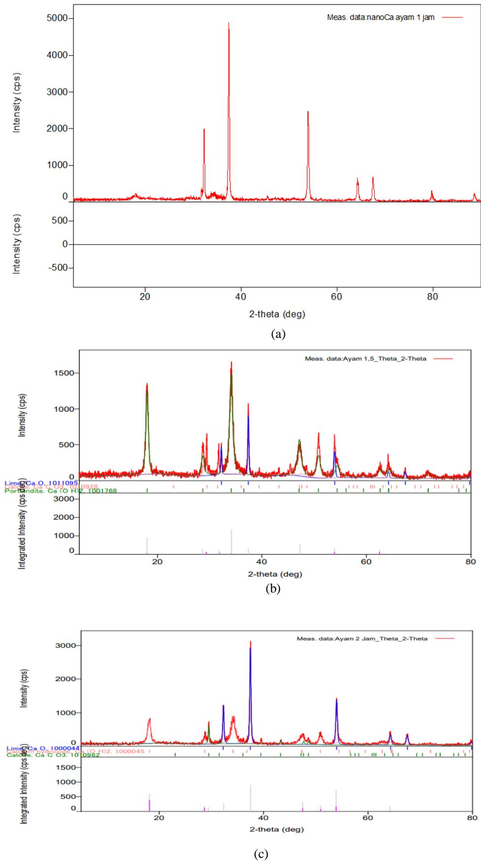
**Figure 2** XRD of nanocalcium chicken eggshells from (a) 1-hour extraction, (b) 1.5-hour extraction, and (c) 2-hour extraction.
