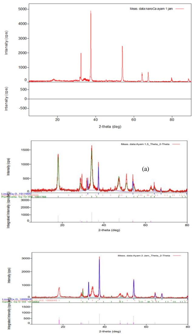
Figure 1 XRD of nanocalcium chicken eggshells from (a) 1-hour extraction, (b) 1.5-hour extraction, and (c) 2-hour extraction.
