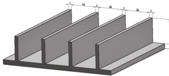
**FIGURE 1.** Geometry and dimension (mm) of the workpiece thin walled Ti<sub>6</sub>Al<sub>4</sub>V
