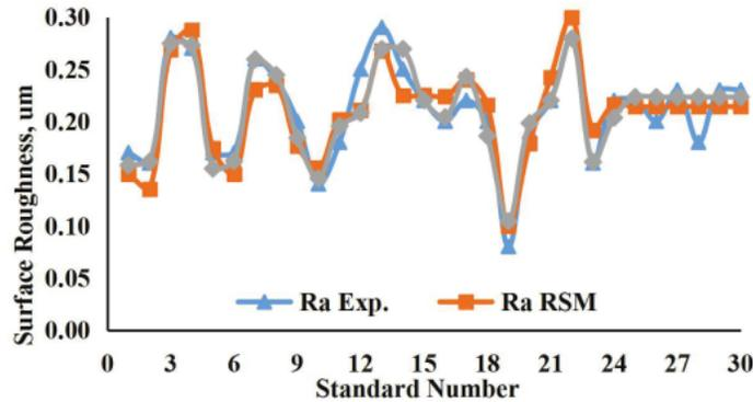
**FIGURE 5.** Surface roughness for experiment and predicted values
